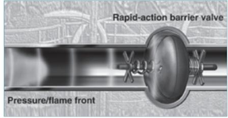
**Figure 8: Explosion isolation with rapid reaction valve**
