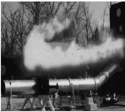
**Figure 6: Explosion venting**
