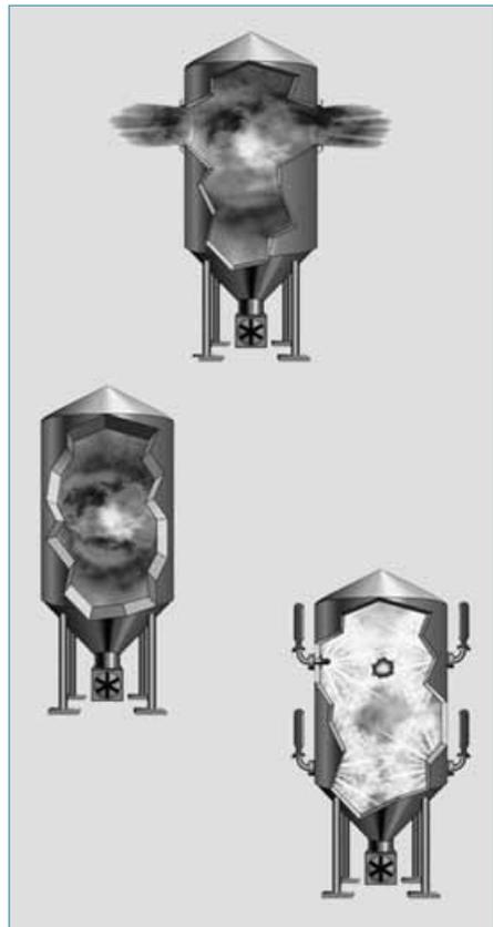
Figure 5: Explosion resistant vessel (left), explosion venting (top) and explosion suppression (bottom right)
